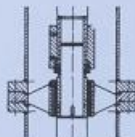
带有中间支承和套筒联轴器 intermediate bearing with split and sleeve-coupled shaft
